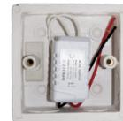
5 Embed the upper touch panel into the baseplate and then tap the bottom to press into the slots.
